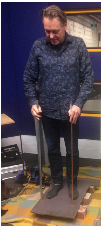
Fig. 2. This sheet of 8mm steel has a transducer attached that can be seen at the back left. The transducer creates vibrations that pass through the body and any other materials that are in contact with the vibrating surface. Dr. Malte Wagenfeld, who was providing critical feedback at this stage of the project, is pictured.
